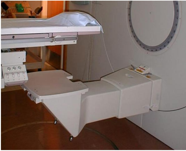
(a) The radiation detector and patients bed. The detector can rotate 360 degrees around the patient so that radiation can be passed through at the appropriate angle.
