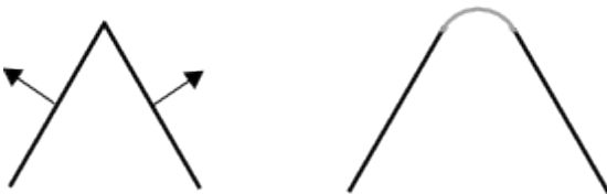
Figure 5: When pieces come apart during propagation, forming a gap, a rarefaction fan must be built.
