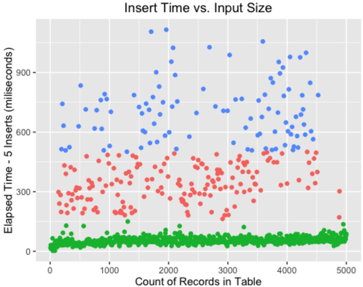
**Figure 22: Visualization of the relationship between the time taken to complete a series of insertions and the input size for the embedded flash implementation of the linear hash. The input size does not affect the time taken for insertions. The blue dots correspond to insertions which trigger a split to occur, the red dots are insertions which required the creation of an overflow bucket, and the green dots required no additional processing.**
