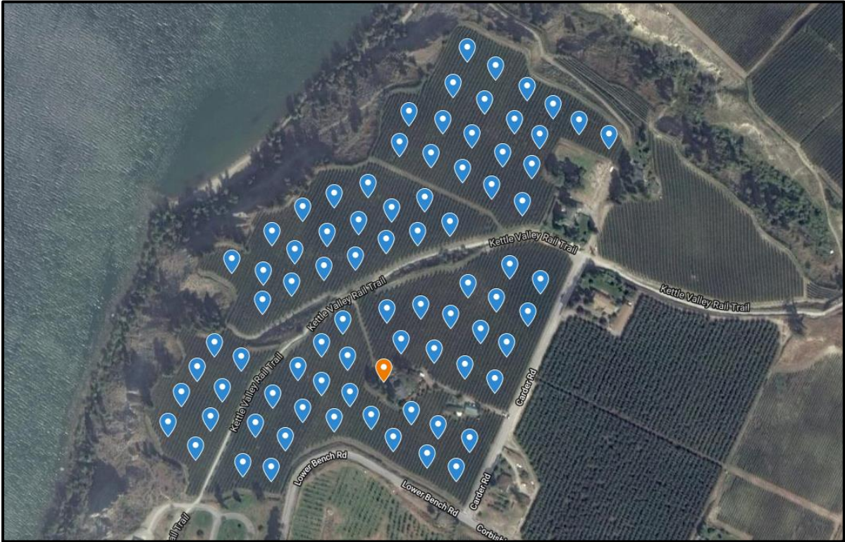
Figure 2: Example layout of a central gateway and sensor nodes in a vineyard
