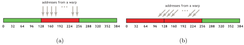
Figure 2.2: A fully coalesced memory access (a) and a sequential but misaligned memory access (b) [4].
