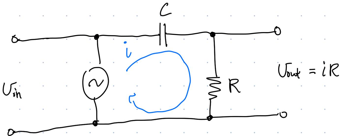
Write  $V_m = V_{in} e^{j\omega t}$        $V_{out} = V_{out} e^{j(\omega t + \phi)}$
