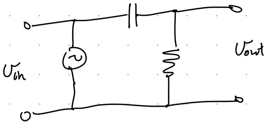
At high freq, no phase ( $\phi = 0$ ) between input and output.
