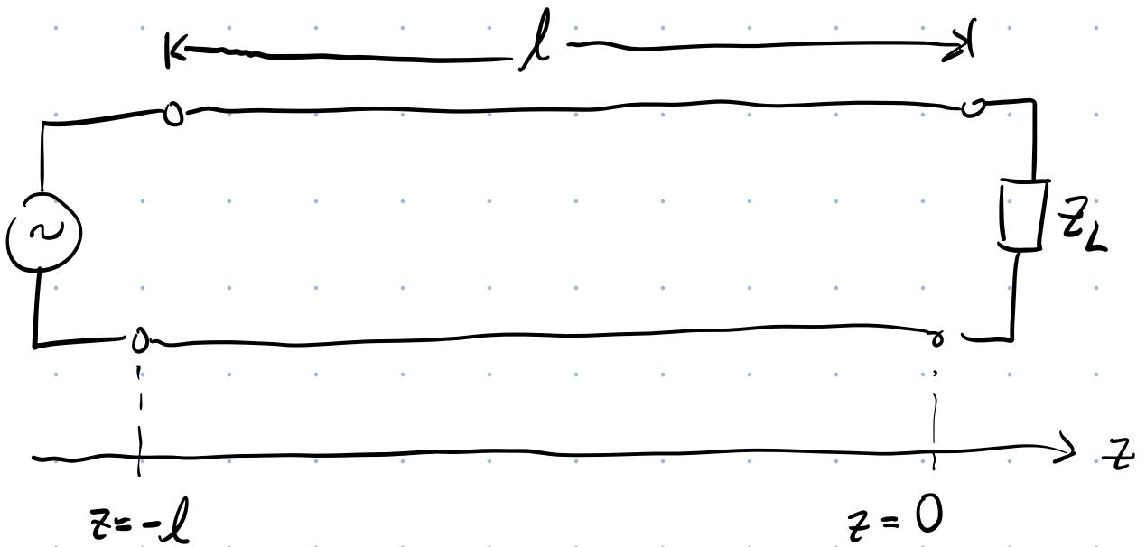
With  $i$ 's choice of coord. sys., the voltage & current amplitudes at the position of  $Z_L$  ( $z=0$ ) are given by:
