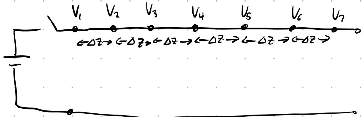
Expect  $V_1 > V_2 > V_3 \dots > V_7$  a short time after switch is closed. Simple LC circuit model fails for long trans. lines b/c can only have one volt. diff. across L.
