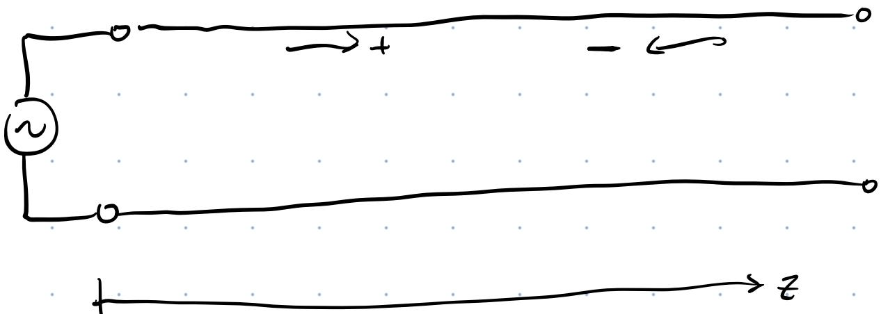
Backwards travelling waves are due to reflections from the opposite end of the transmission.
