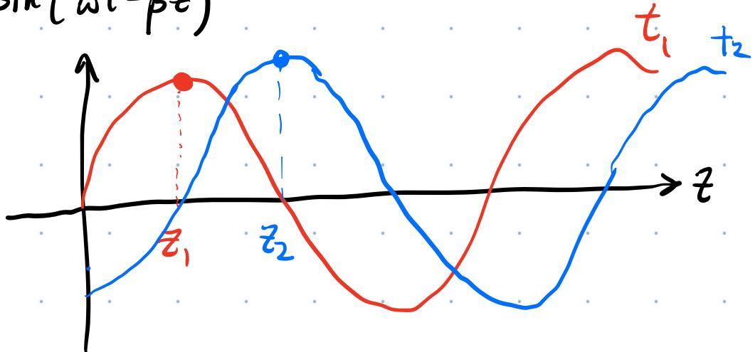
Require:  $\sin(\omega t_1 - \beta z_1) = \sin(\omega t_2 - \beta z_2)$
