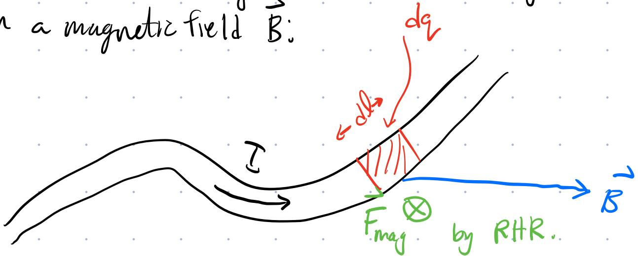
$$\vec{dF}_{\text{mag}} = \underbrace{dq \vec{v} \times \vec{B}}_{\lambda dl} = \underbrace{(\lambda \vec{v}) \times \vec{B} dl}_{\vec{I}}$$
