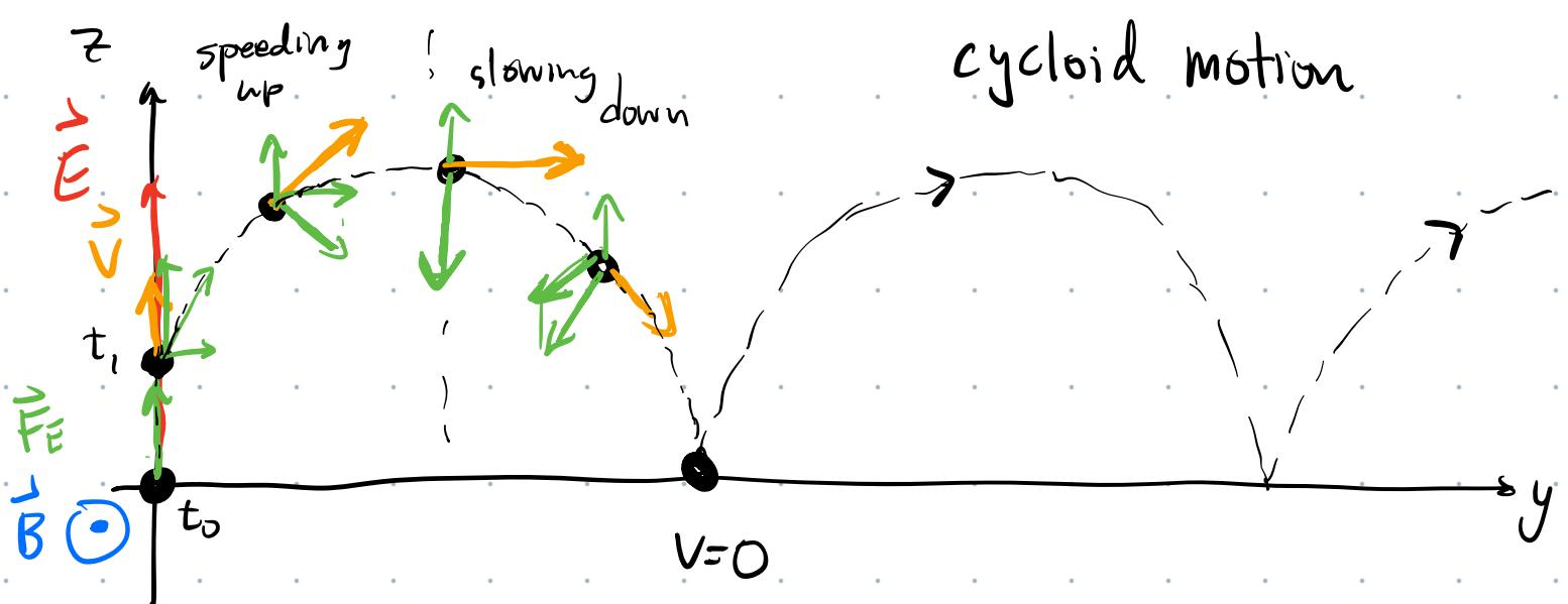
Motion of  $q$  is  $\perp$  to both  $\vec{E}$  &  $\vec{B}$ .
