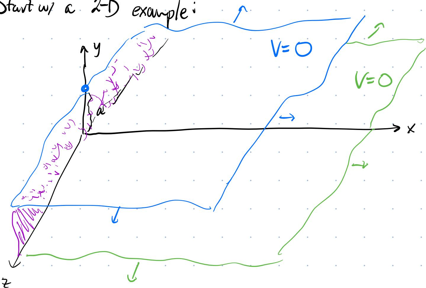
Two parallel semi-infinite conducting sheets both at  $V=0$ . One sheet is in  $xz$ -plane. The other is at  $y=a$ .
