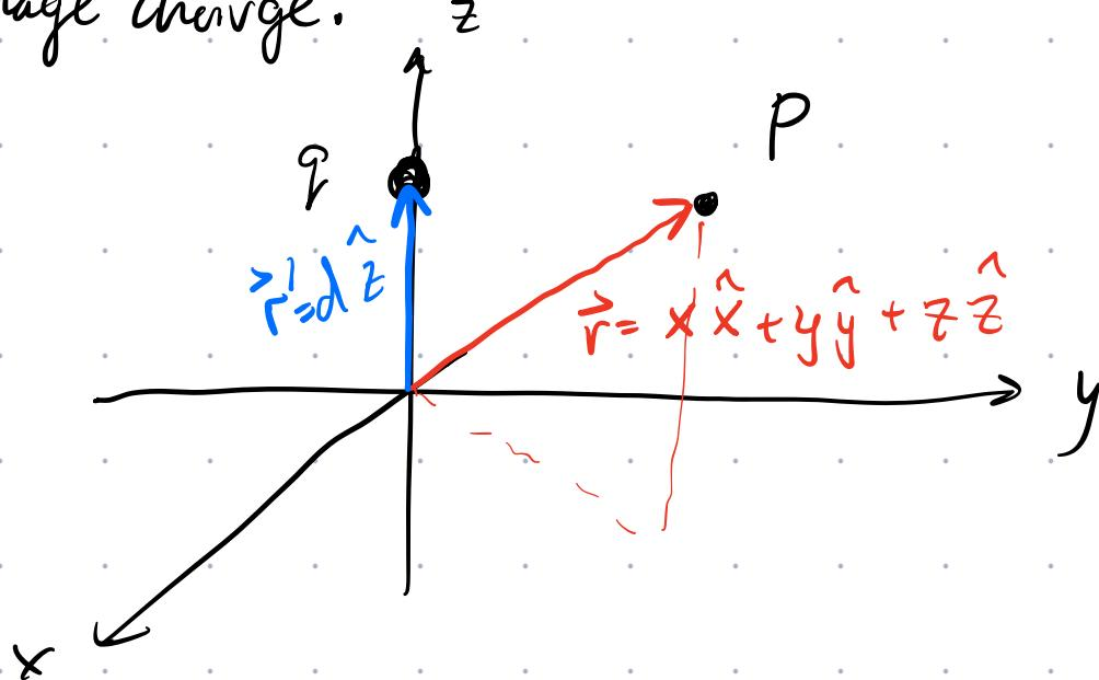
For pt. charge  $V_+ = \frac{1}{4\pi\epsilon_0} \frac{q}{R_+}$
