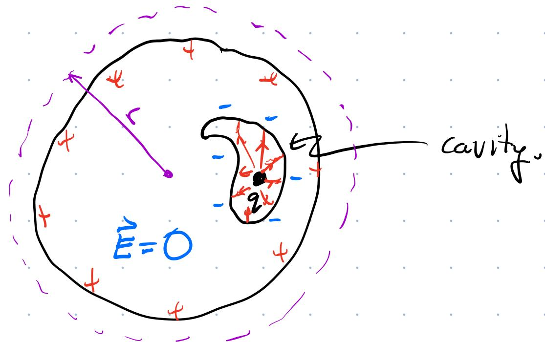
Put a pt. charge  $q$  inside cavity at arbitrary position.
