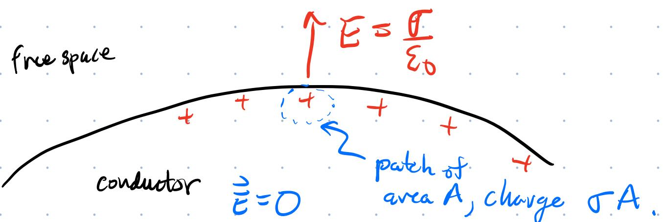
Conductor w/ surface charge density  $\sigma$ .
