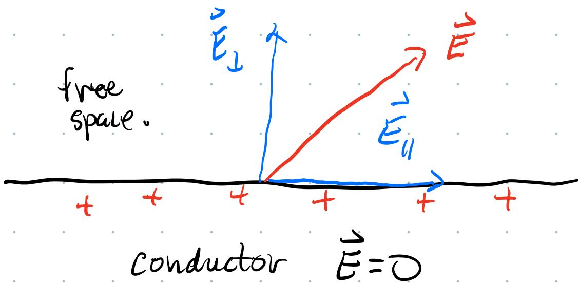
A charged conductor in an external  $\vec{E}$ -field.
