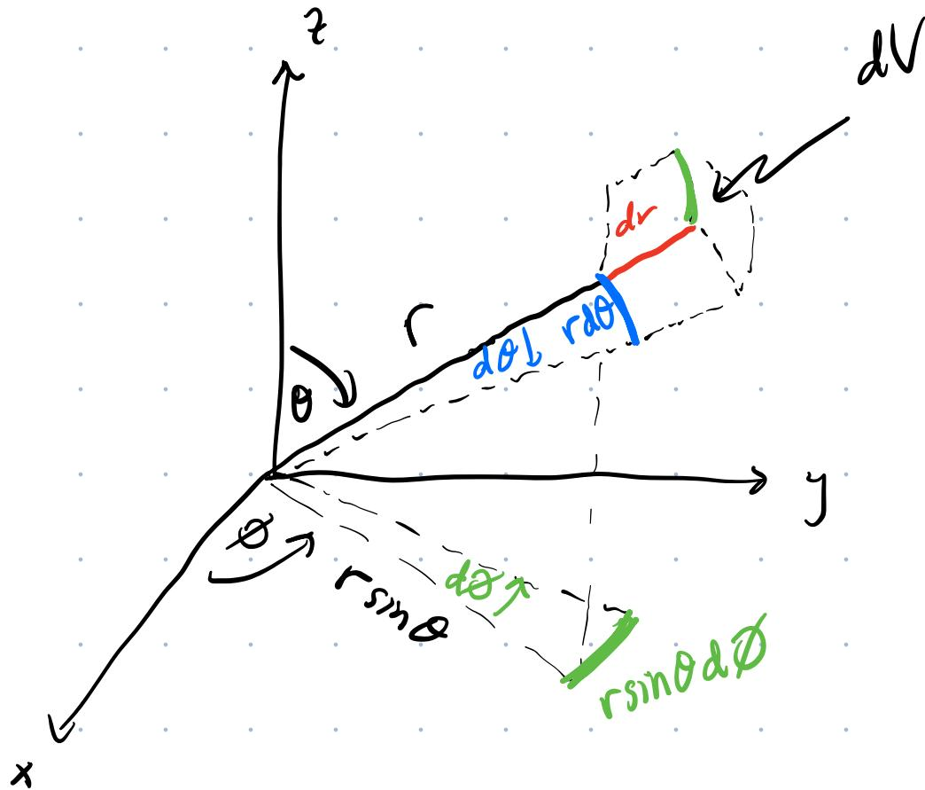
$$\begin{aligned} dV &= (dr)(rd\theta)(rsin\theta d\phi) \\ &= r^2 sin\theta dr d\theta d\phi \end{aligned}$$
