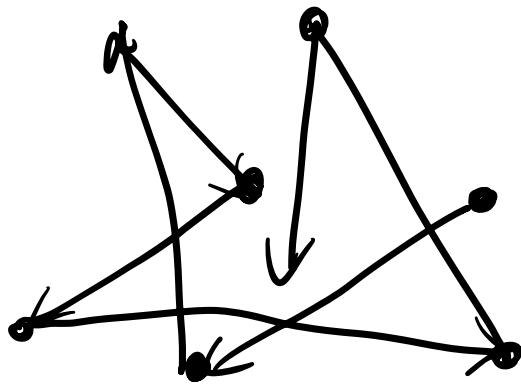
here  $l$  is the avg. distance traveled by particle between scattering events.  $l$  is called the "mean free path".
