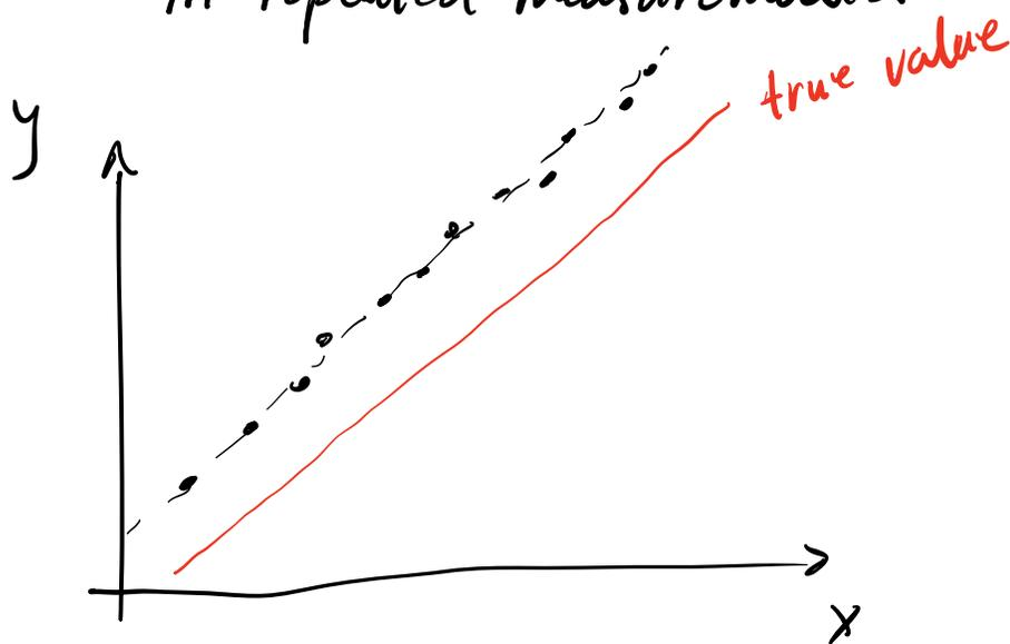
A precise, but inaccurate measurement.
