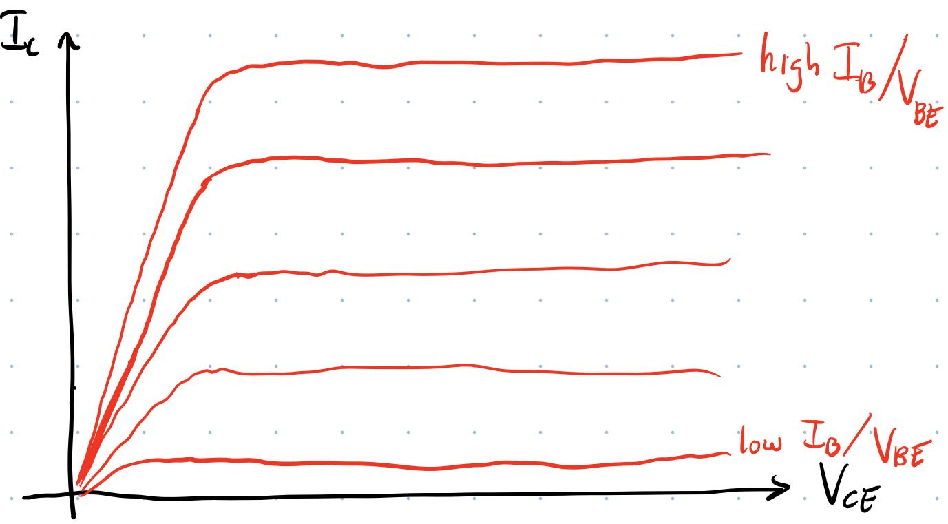
At some pt., essentially all  $e^-$  reach the collector  $\{\}$  increasing  $V_{CE}$  no longer changes  $I_c$ .
