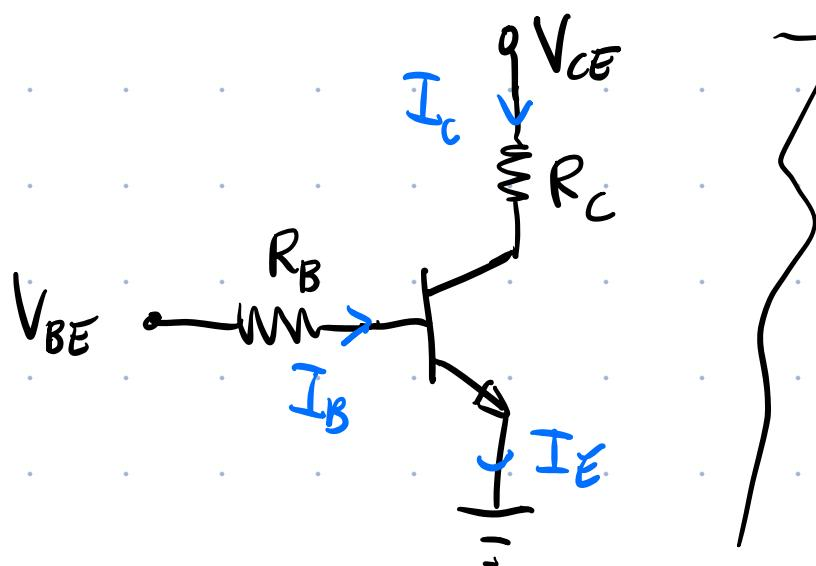
Because the base is thin, most  $e^-$  from emitter cross into the collector.  $\therefore I_B$  is always small.
