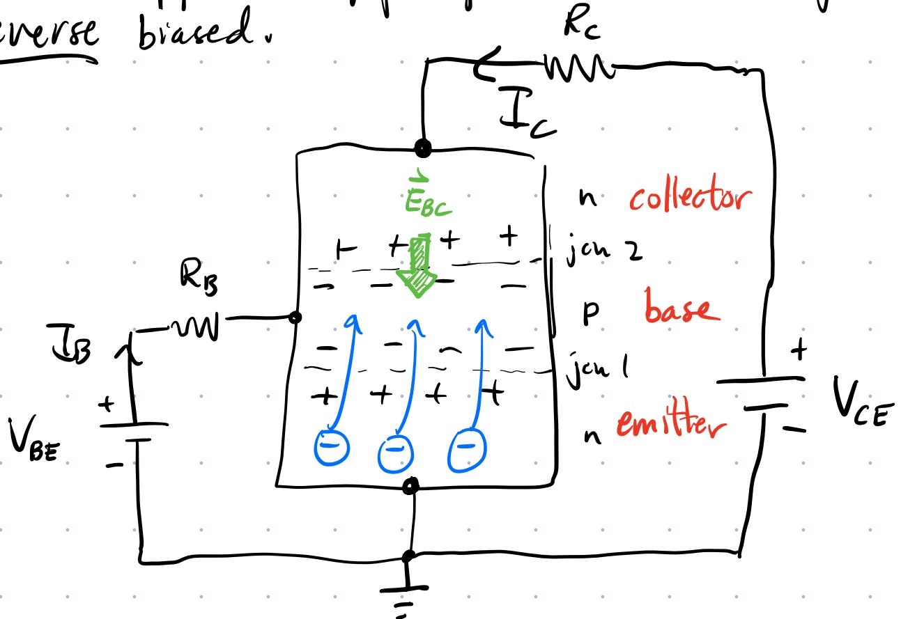
Electrons from emitter injected into the base. Those that reach the depletion region of the base-collector are swept across the jcn by  $E_{BC}$ . The base of the transistor is made thin to increase the prob. that  $e^-$  reach the base-collector jcn.
