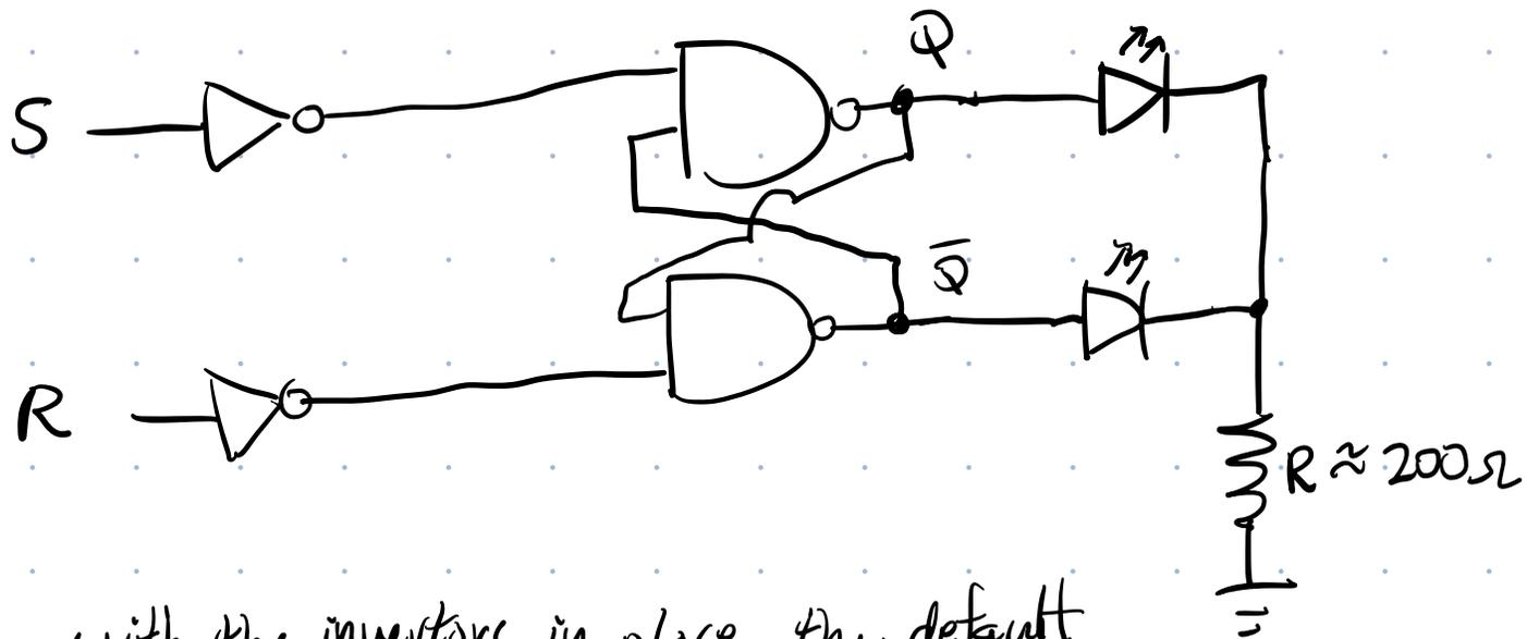
With the inverters in place, the default state of the input is  $(S, R) = (0, 0)$ .
