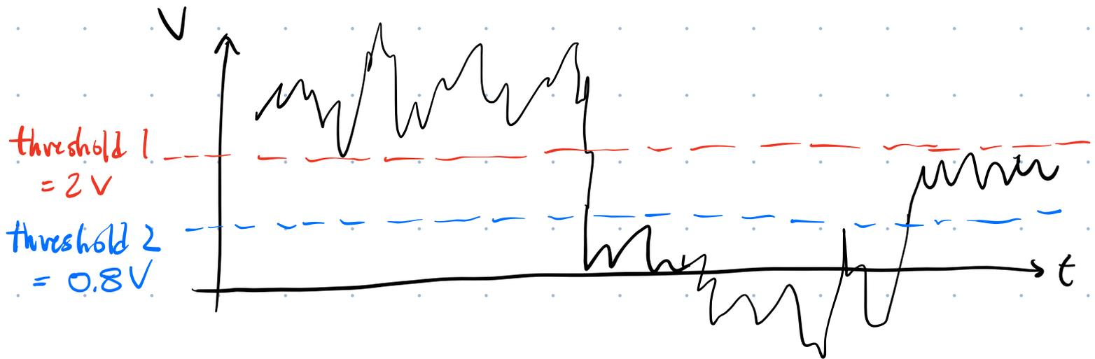
Voltage signal w/ large fluctuations.
