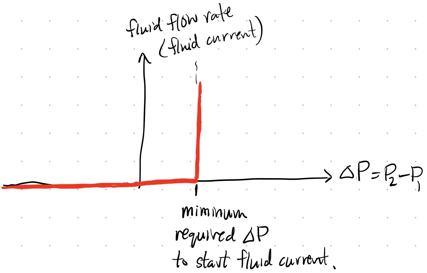
In electronics diodes act as a oneway valve of electric current.
