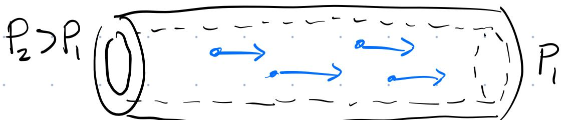
To flow fluid through a pipe, need to establish a pressure difference across pipe.
