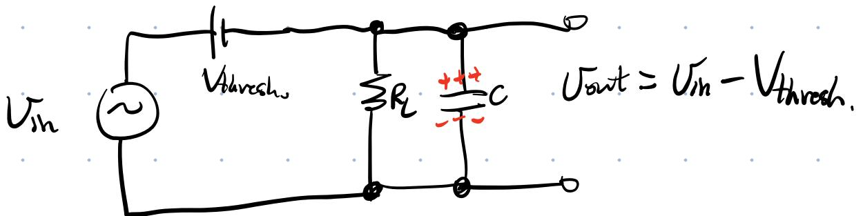
Cap. C charges to  $V_{out}$  while diode is forward biased ( $I \neq 0$ ).
