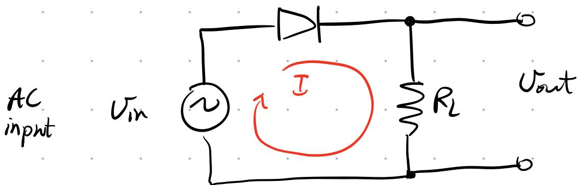
If  $V_{\text{in}} < V_{\text{thresh.}}$ ,  $I = 0$ ,  $V_{\text{out}} = 0$  reverse biased
