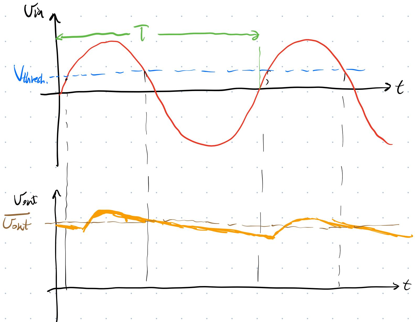
With the cap. in place,  $\overline{V_{out}}$  increases & looks more like a constant DC voltage.
