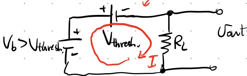
Loop analysis  $V_b - V_{\text{thresh.}} - IR_L = 0$
