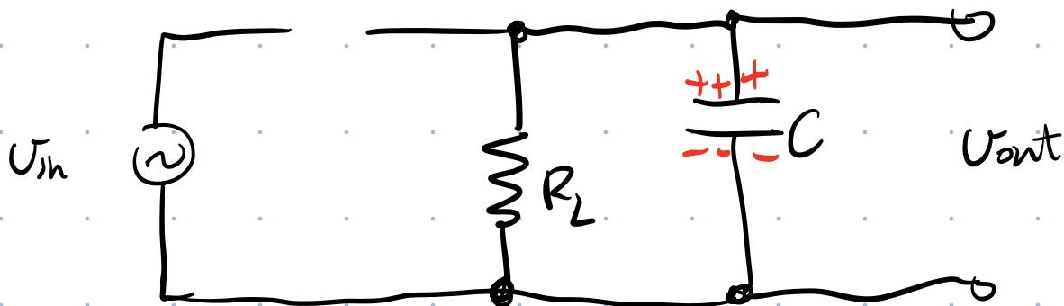
Now, the cap. C discharges through  $R_L$  with a time constant  $\tau = R_L C$
