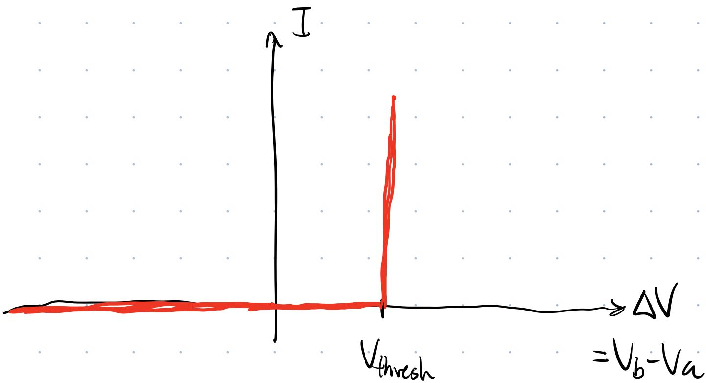
Reverse-biased diode     $V_b - V_a < V_{\text{thresh.}}$
