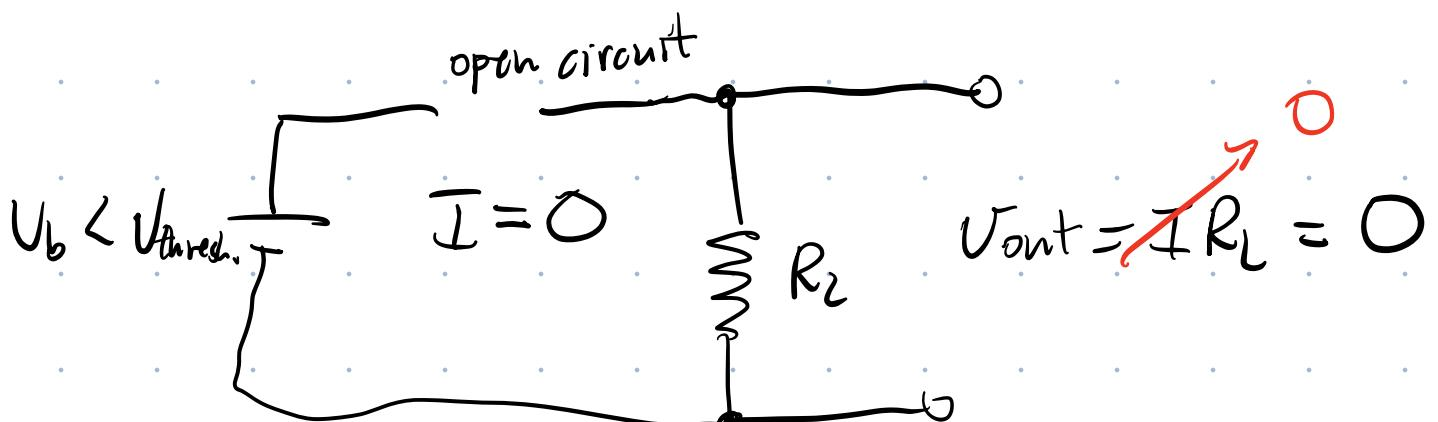
A reverse-biased diode is equiv. to an open circuit.
