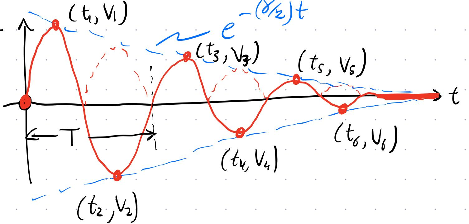
Plot of  $|V_j|$  vs  $t_i$   $\rightarrow$  use the data to meas.  $\gamma$
