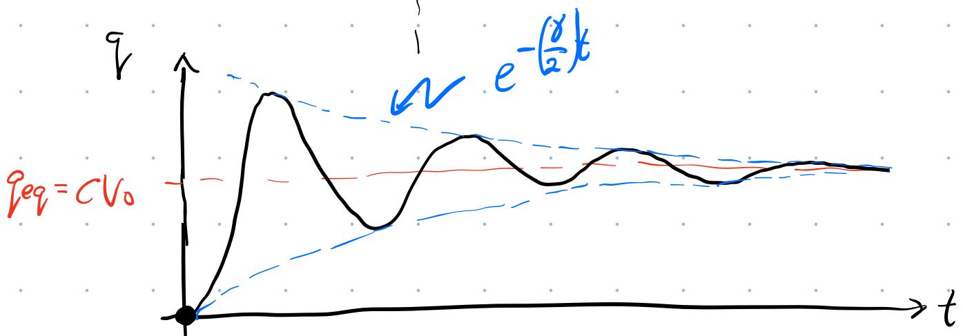
If  $q=0$  @  $t=0$  (initial condition), then for an underdamped LRC circuit ( $R$  small), the sol'n for charge on the cap. as a fn of time is:
