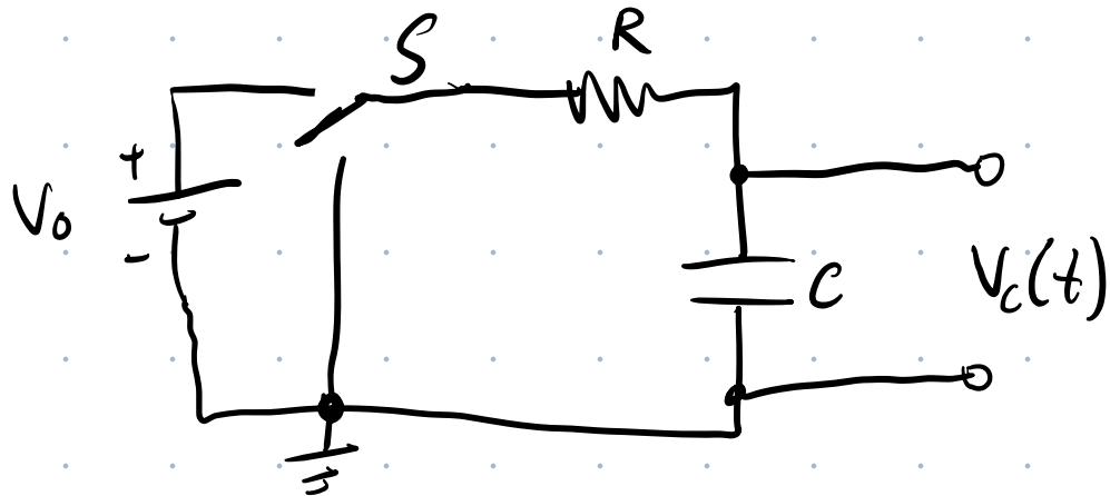
Use square wave TTL output of fcn generator to simulate opening & closing of switch.
