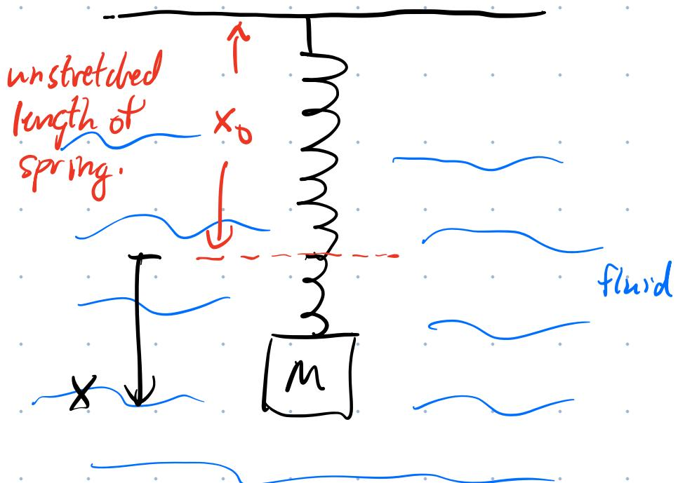
If we stretch & release the mass, it will begin to oscillate about an equil. position. The drag force on the mass due to fluid converts some of the system's mechanical energy into heat. This dissipation, causes the amplitude of the osc. to decrease w/ time (damping).
