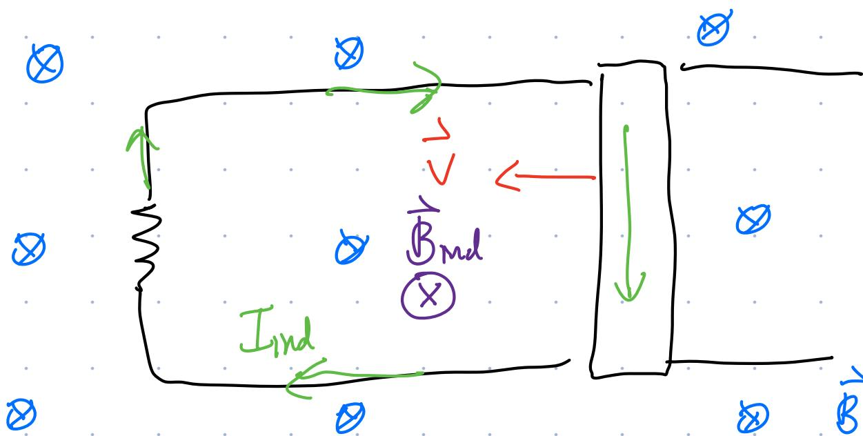
In this case, by RHR par. charge deflected towards btm of rod  $\rightarrow$   $I_{\text{ind}}$  is in CW dir'n.
