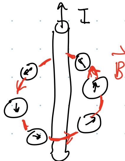
If we reverse the dir'n of  $I$ , the magnetic field changes dir'n as well (i.e. the rotate by  $180^\circ$ ).
