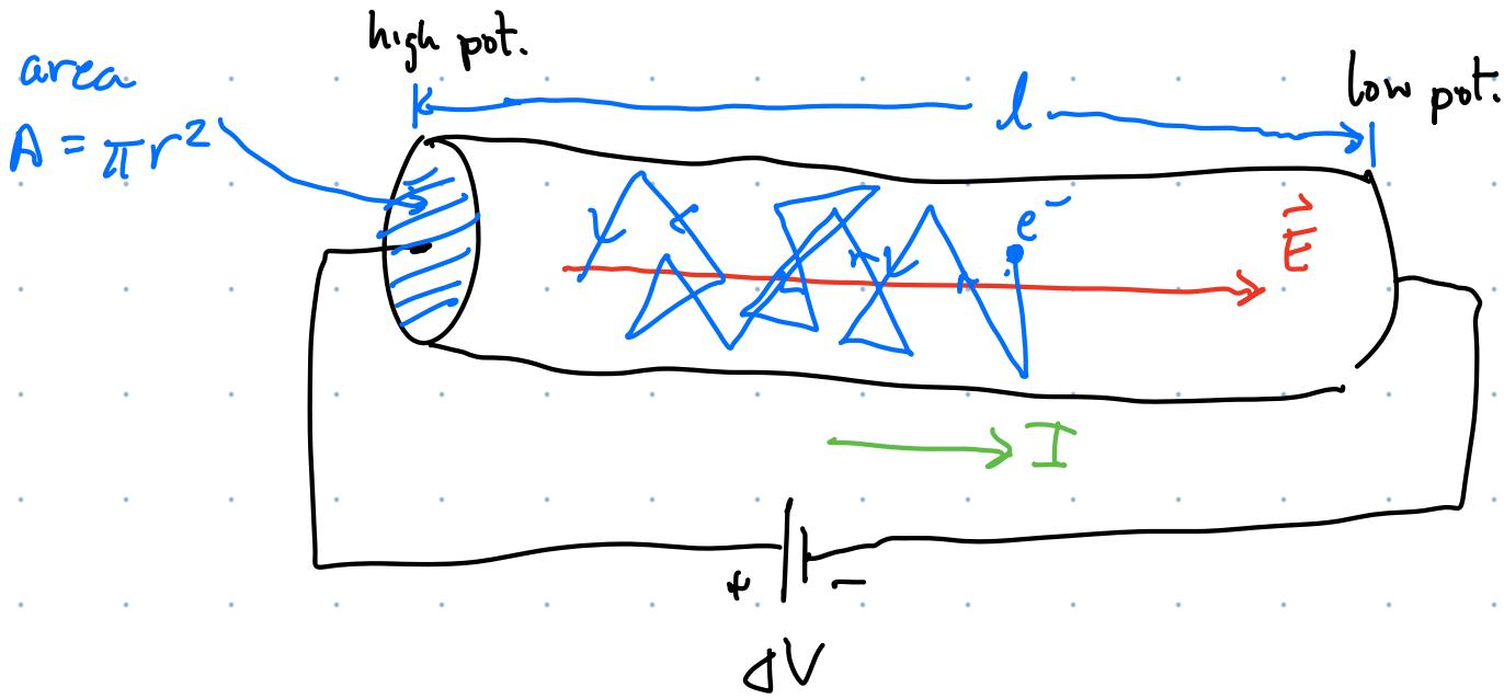
Pot. diff. across wire, establishes an  $\vec{E}$  in the wire which exerts a force on conduction  $e^-$ . This force cause a slow drift of  $e^-$  from right to left.
