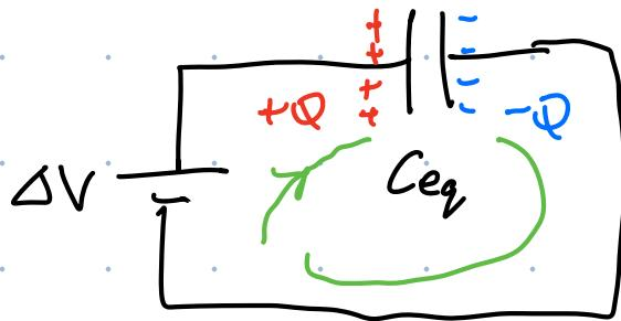
loop rule:  $+ \Delta V - \Delta V_{C_{eq}} = 0$
