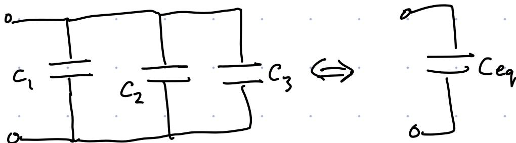
$$C_{eq} = C_1 + C_2 + C_3$$
