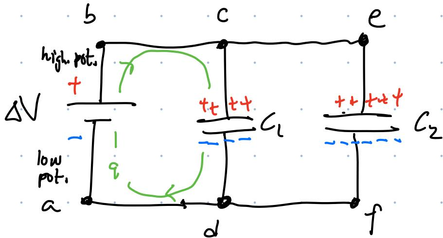
Imagine taking a charge  $q$  around any closed loop in the circuit.
