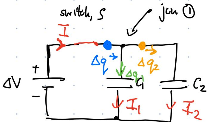
When we close the switch, got a flow of charge or a current that transports pos. charge from the btm plates to the top plates.
