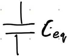
Want to represent the parallel comb. as a single "equivalent" capacitor  $C_{eq}$ .
