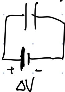
$$\frac{1}{C_{eq}} = \frac{1}{C_1} + \frac{1}{C_2} + \frac{1}{C_3}$$
