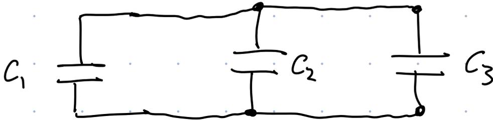
All top plates connected by a wire } Parallel
