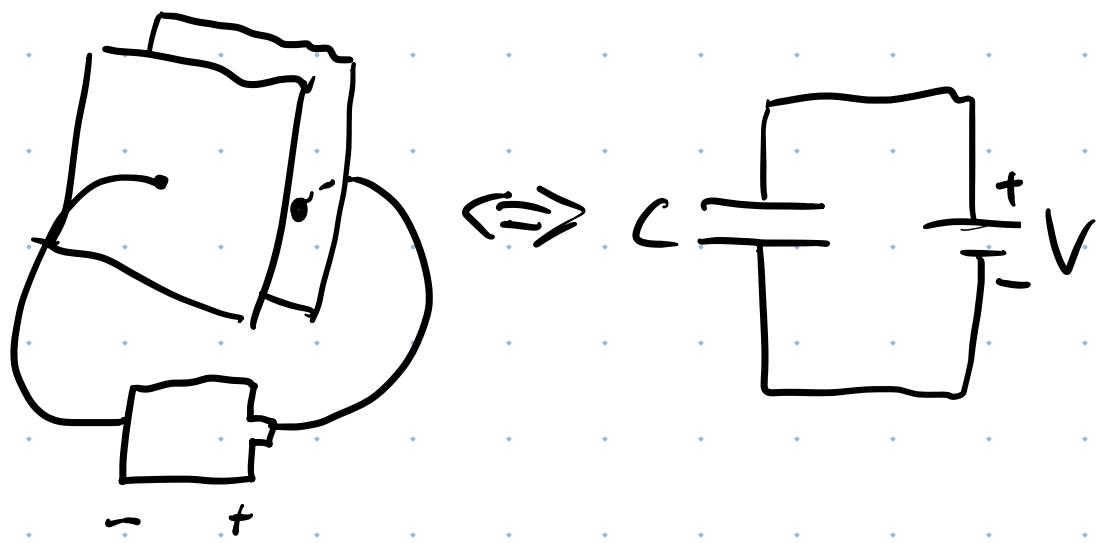
Eg. A parallel plate cap. is connected to a battery of voltage  $\Delta V$ . The charge on the plates is  $\pm Q_1$ .
