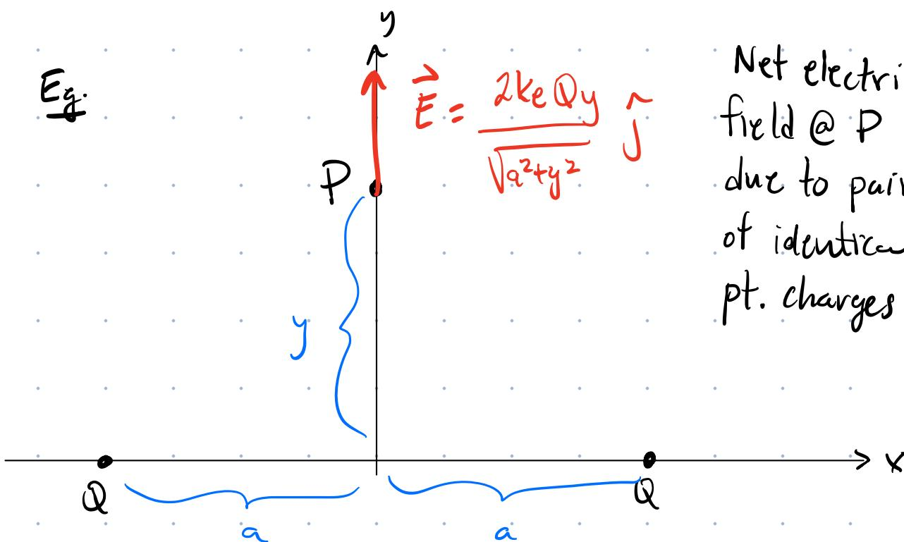
Net electric field @ P due to pair of identical pt. charges  $Q$
