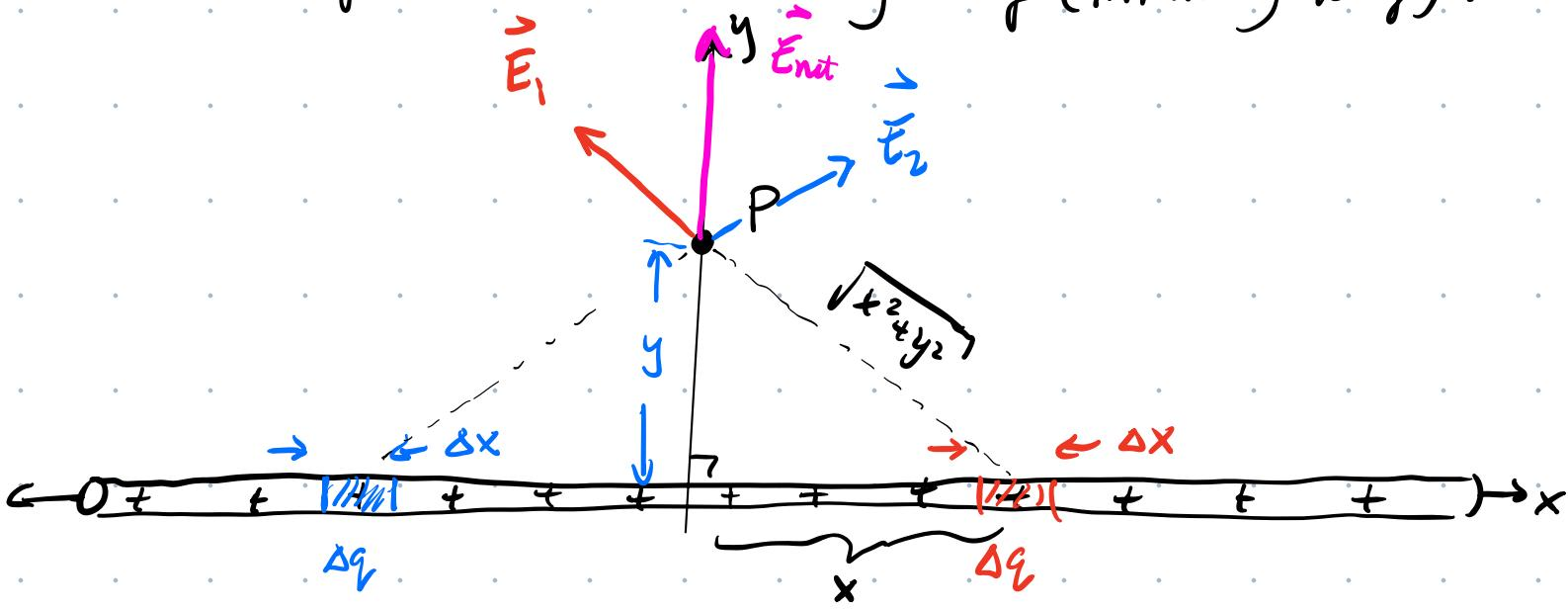
Select a section of rod of length  $\Delta x$  (small). That section of rod has charge  $\Delta q$ , which we treat as a pt. charge.  $\Delta q$  contributes an electric field  $\vec{E}_1$  @ pt. P.
