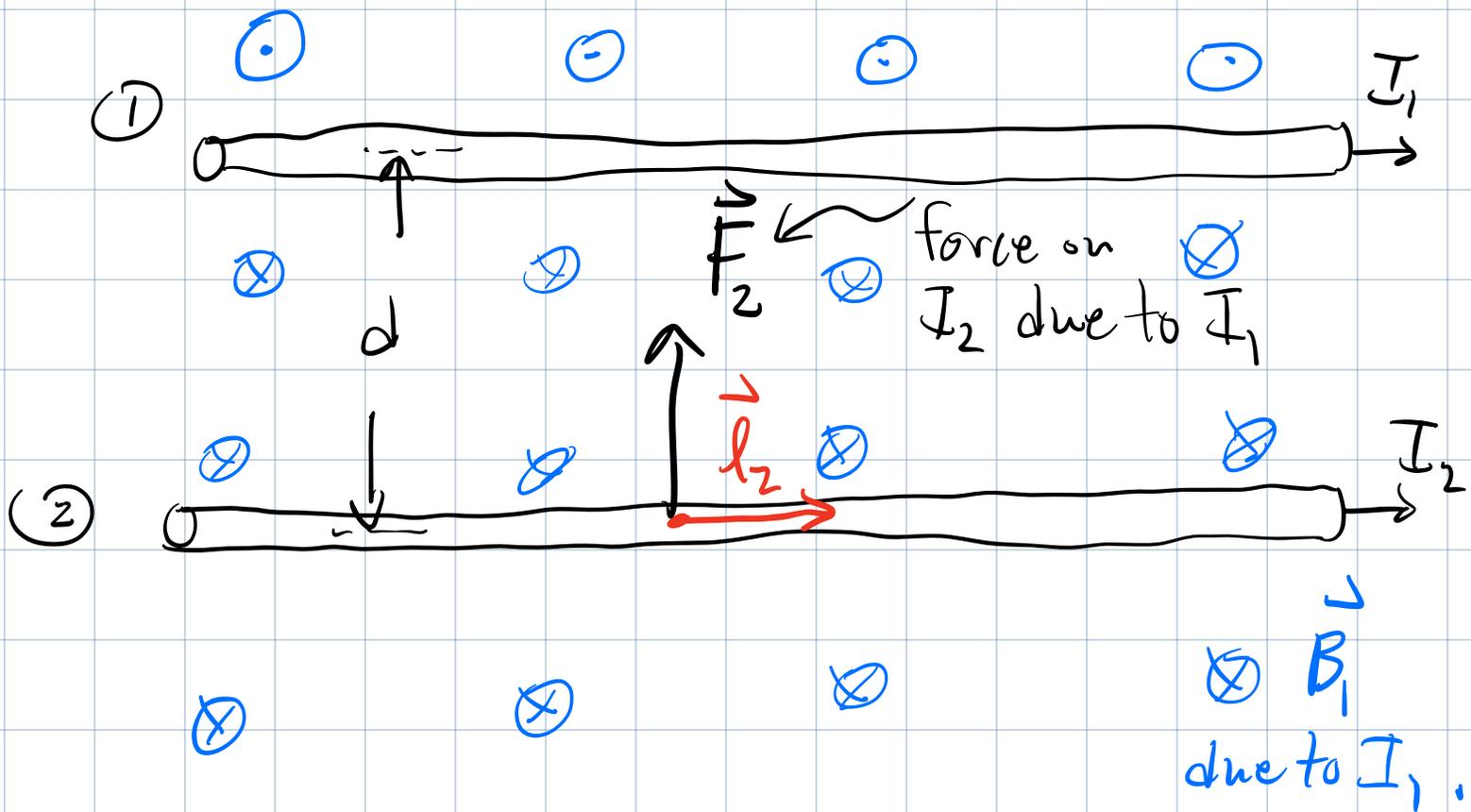
What is the force on  $I_2$  due to magnetic field of  $I_1$ ?
