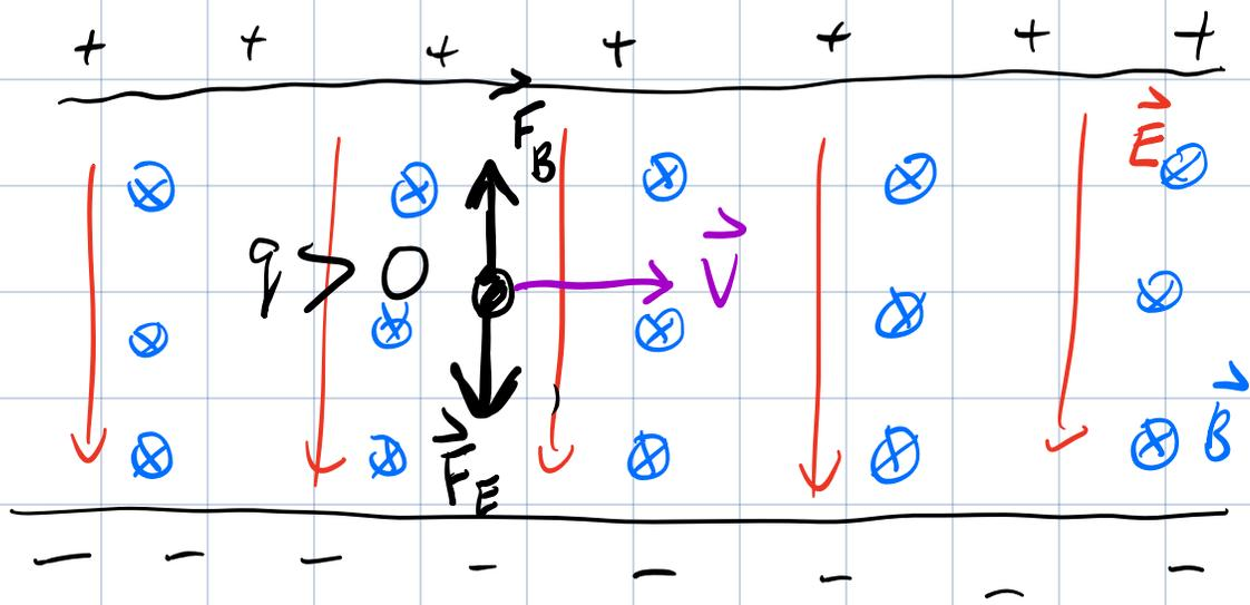
Next, apply a uniform magnetic field  $\vec{B} \perp$  to  $\vec{E}$ .
