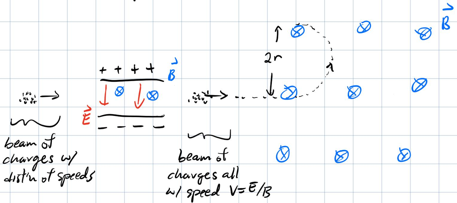
After charges leave velocity selector, they enter a uniform magnetic field  $\vec{B}$  w/  $\vec{v} \perp \vec{B}$  & undergo circular motion w/ radius
