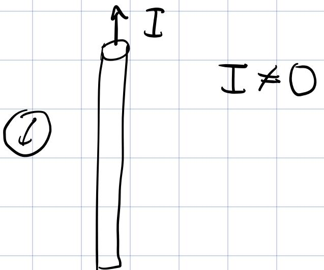
The current in the wire creates a magnetic field that deflects the compass needle.
