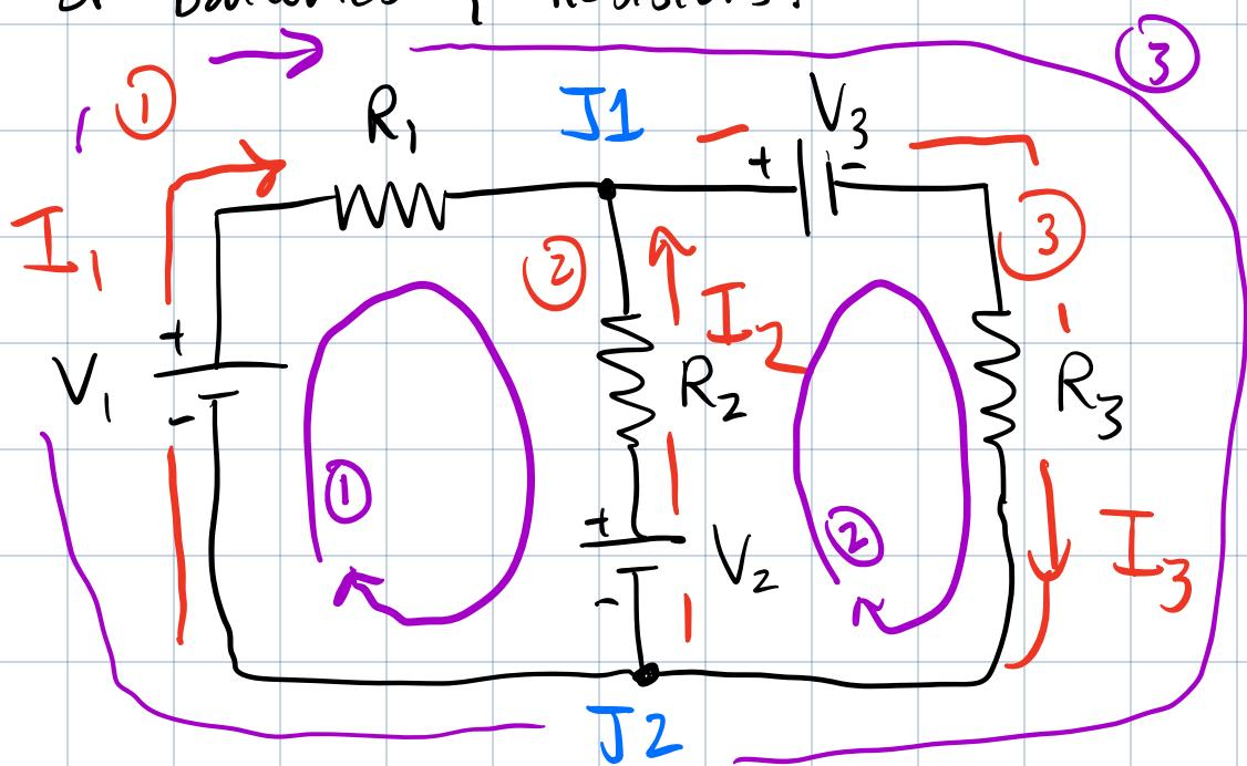
Typically in a circuit like this will have some unknowns to solve for (currents, battery voltage, resistor values)
