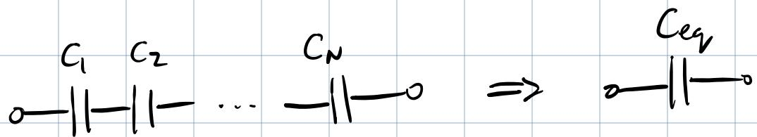
$$\frac{1}{C_{eq}} = \sum_{i=1}^N \frac{1}{C_i} = \frac{1}{C_1} + \frac{1}{C_2} + \dots + \frac{1}{C_N}$$
