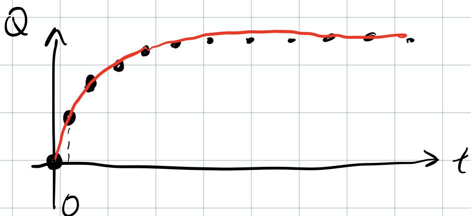
After a short time  $\Delta t$ , capacitor accumulates some charge  $\Delta Q = I \Delta t$
