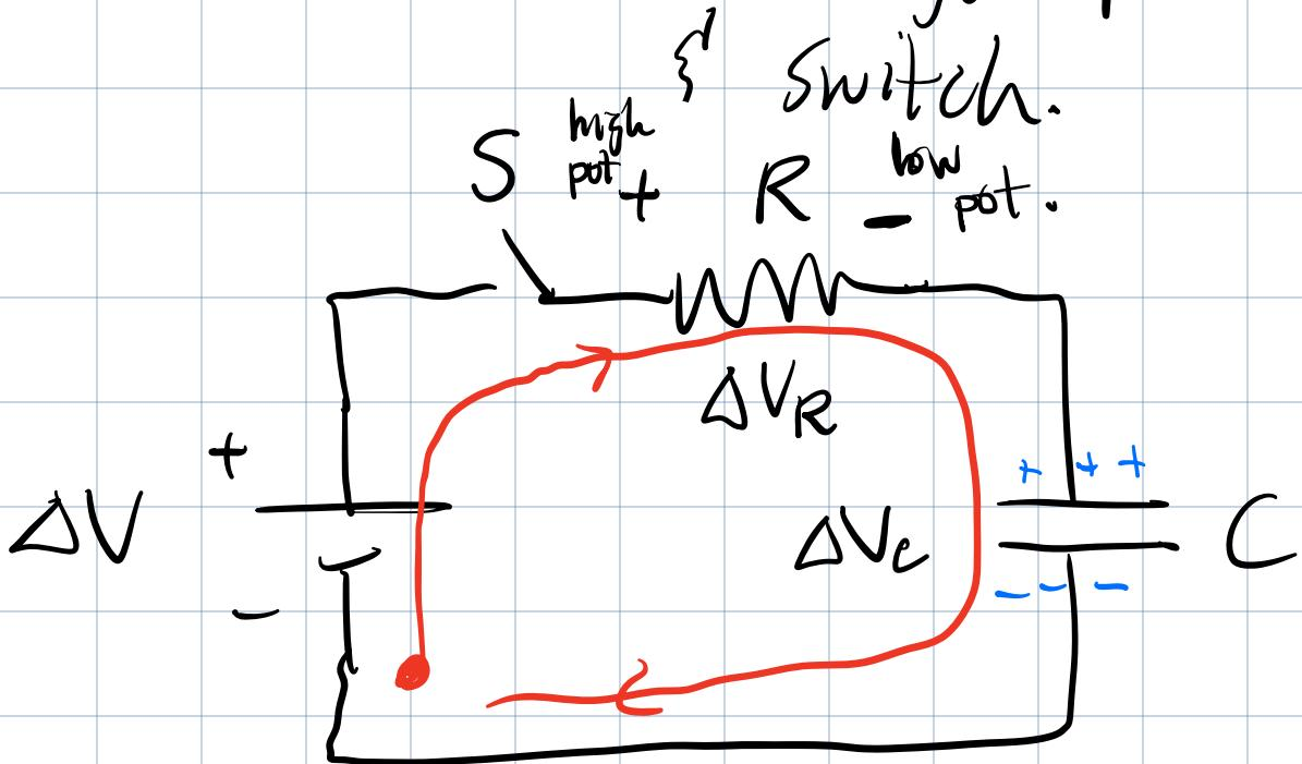
If  $C$  is initially uncharged { switch  $S$  is closed at time  $t = 0$ .
