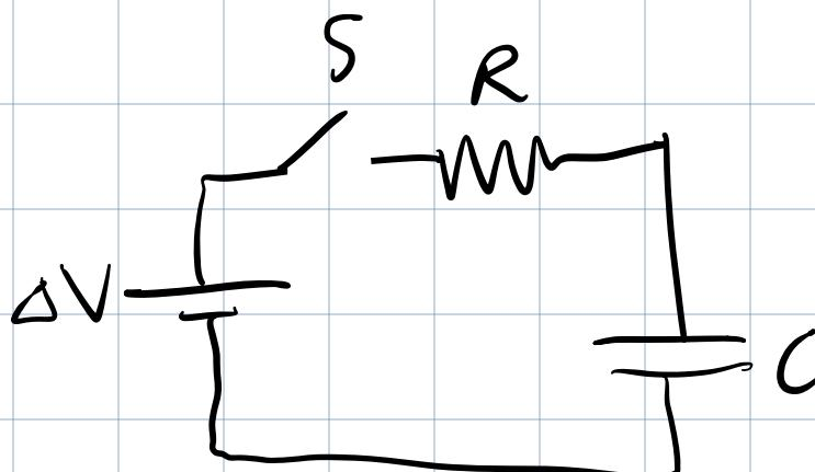
If  $S$  is just closed  $\Delta V_C = 0$  (initially uncharged)
