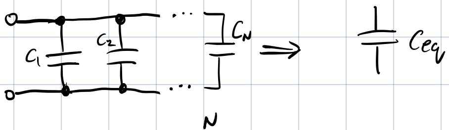
$$C_{eq} = \sum_{i=1}^N C_i = C_1 + C_2 + \dots + C_N$$
