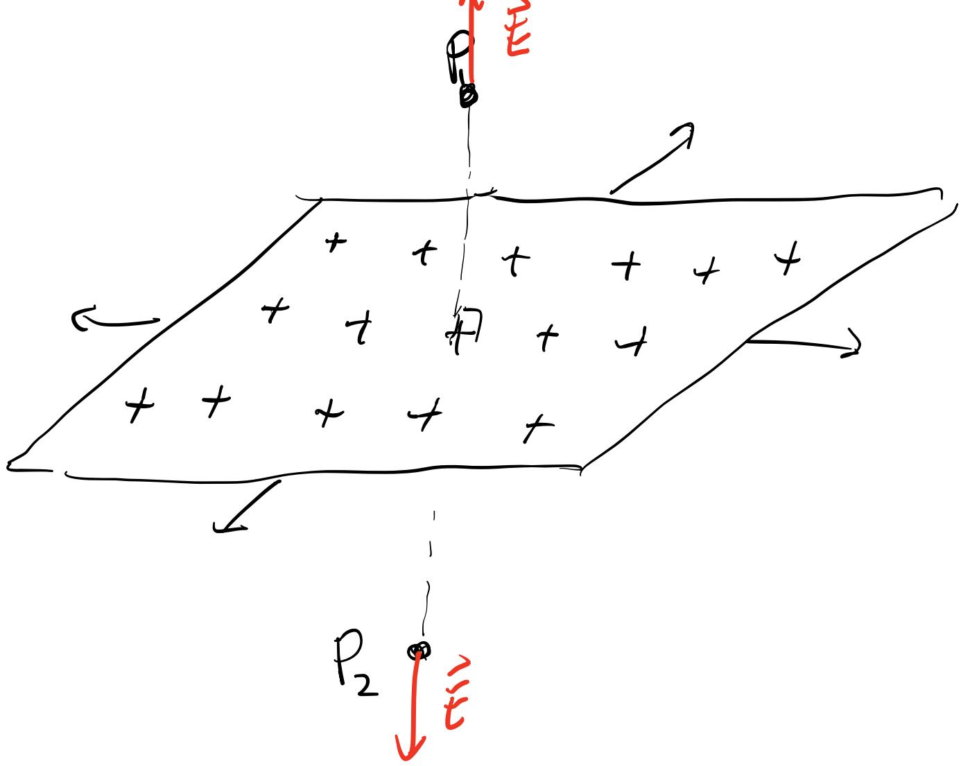
By symmetry  $\vec{E}$  anywhere above sheet is upwards & it is downwards below the sheet.
