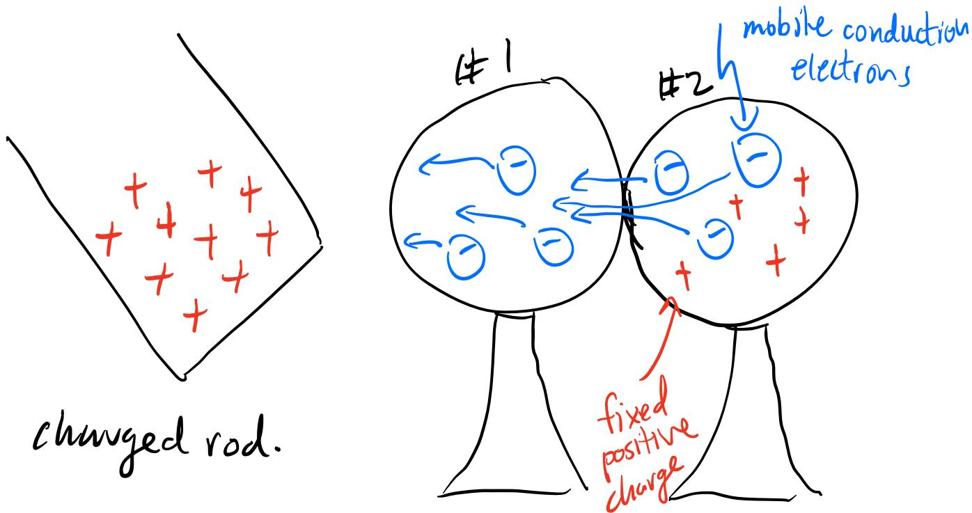
The positively-charged rod attracts mobile conduction electrons. Therefore, there is a migration of electrons from conductor #2 to conductor #1. This process leaves behind an excess positive charge on #2 due to fixed positive nuclei.
