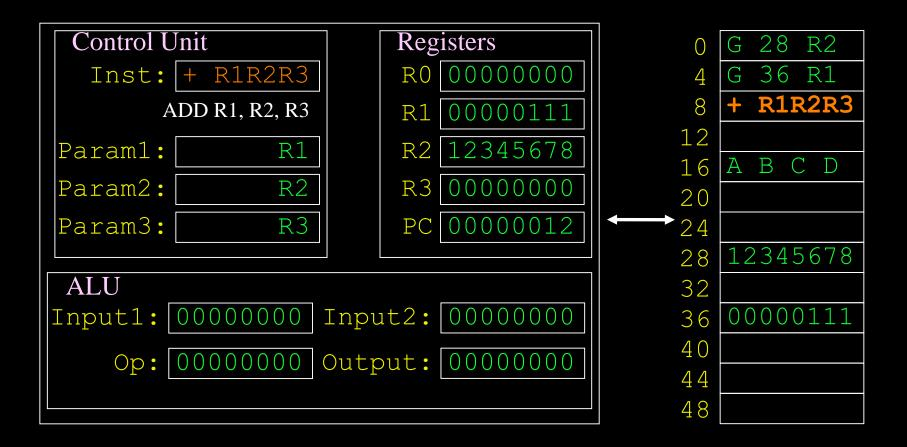
Decode instruction to determine it is an add. Set param1 to R1 (register 1), param2 to R2 (register 2), and param3 to R3 (register 3). Prepare ALU to receive command and inputs. COSC 122 - Page 23
