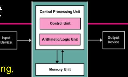
• arithmetic/logic unit (ALU) – responsible for performing mathematical functions (addition, subtraction, etc.) and logical operations (AND, OR, NOT)
