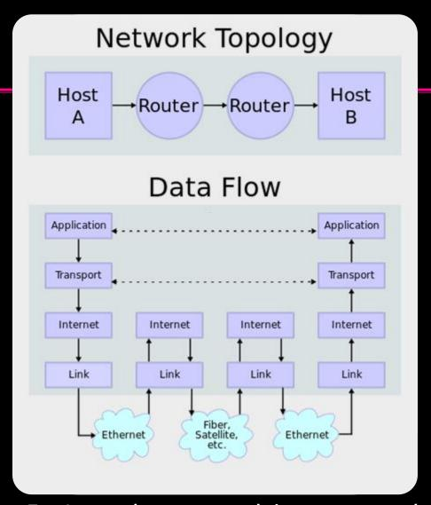
Two Internet hosts connected via two routers and the corresponding layers used at each hop.
